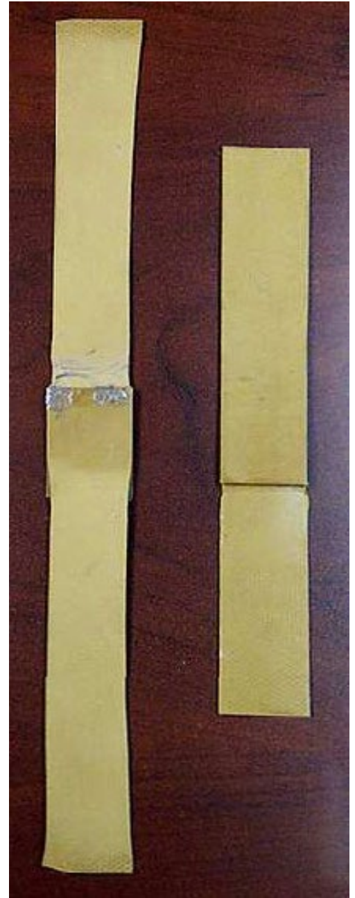
[Figure 1] – The Rulon J sample on the left was subjected to plasma treatment and bonded.
