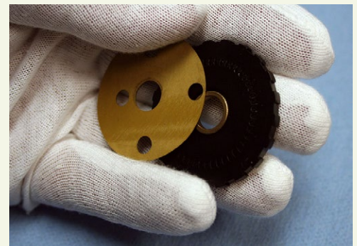
Rulon LR and J materials used in slip-clutch assembly.
