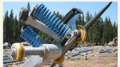
Pivot point bearings on grip cable jaws
